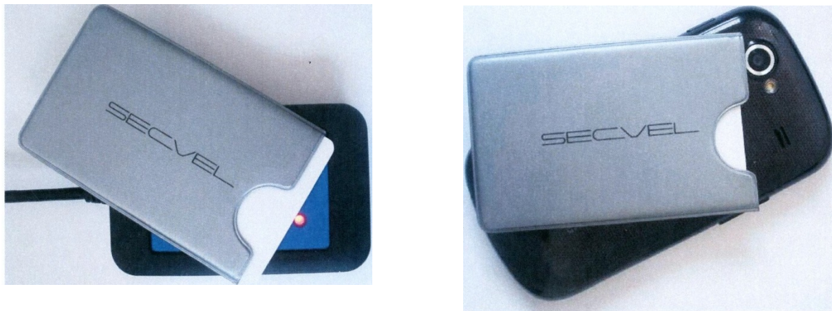
Fig. 1.2: Configurations (depth of card insertion) in which RFID access was still possible in the case of contact with the reader or smart phone.
