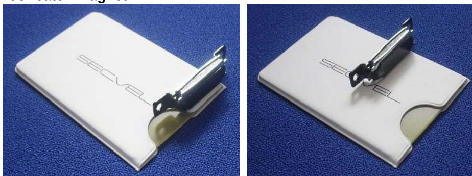
Fig. 5.3: Position of the pinboard magnets and door catch magnet on the SECVEL Card Protection Sleeve during measurement of the magnetic field inside the sleeve.
