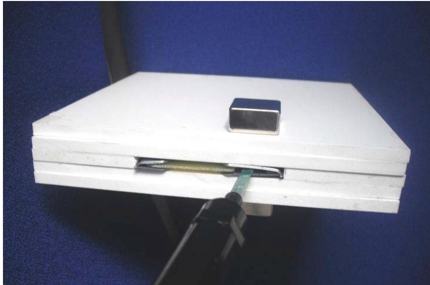
Fig. 5.2: Measuring setup to determine the extent to which the device under test weakened an external magnetic field in the vicinity of the magnetic stripe.
