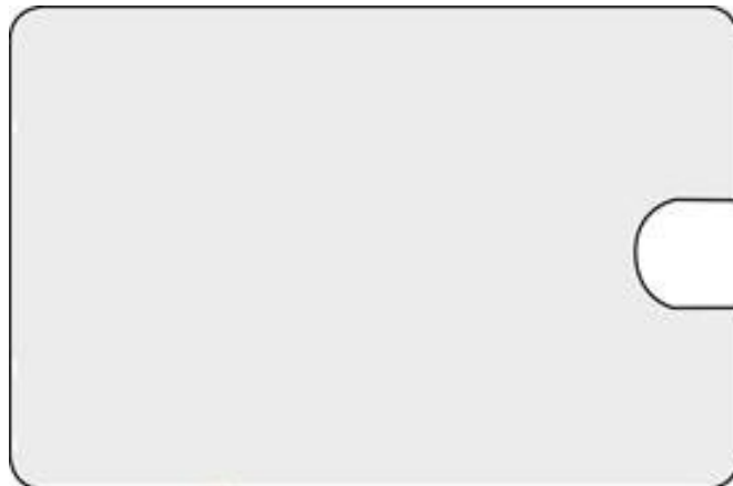
Fig. 7.3: Outline of an improved design SECVEL Card Protection Sleeve with regard to covering the magnetic stripe, whereby the improper insertion shown in Fig. 7.2 is no longer possible and therefore better protection of the magnetic stripe can be achieved in practice.
