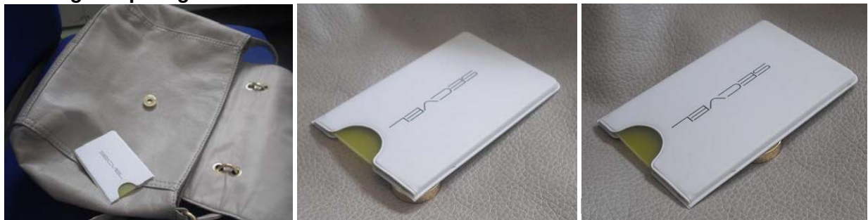
Fig. 5.5: Position of the handbag clasp magnets on the SECVEL Card Protection Sleeve during measurement of the magnetic field inside the sleeve (only one of the three handbags pictured).
