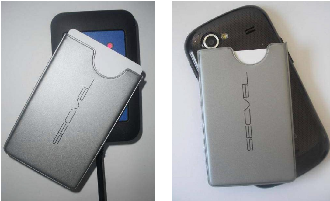
Fig. 5.8: Examples of scenarios used to investigate the extent to which incomplete insertion of cards into the SECVEL Card Protection Sleeve undermines the field weakening effect of the sleeve. Left: tests with a RFID desktop reader. Right: tests with a smart phone with NFC interface.
