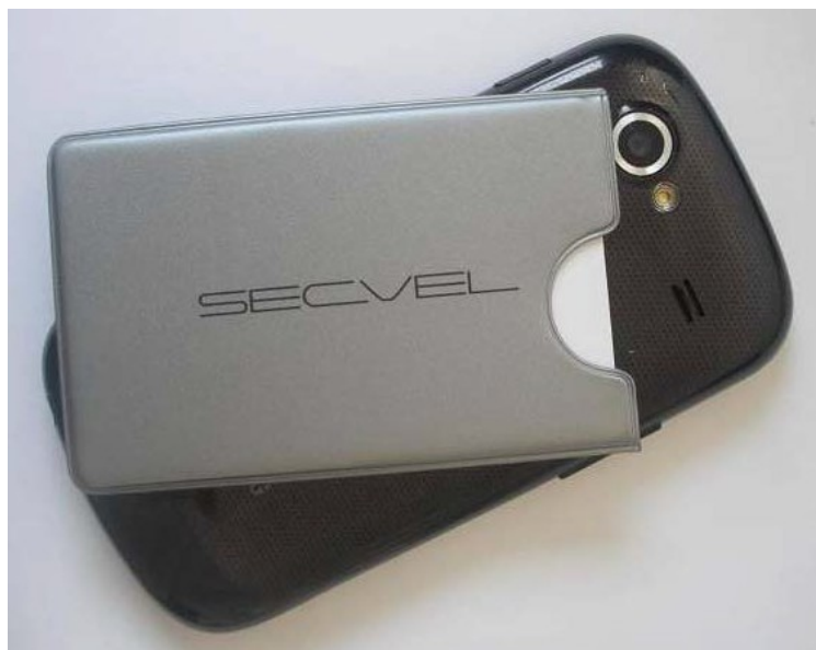
Fig. 7.5: Even with a card fully inserted into the SECVEL Card Protection Sleeve it was still possible to read the card with the smart phone used when the smart phone was touching the surface.
