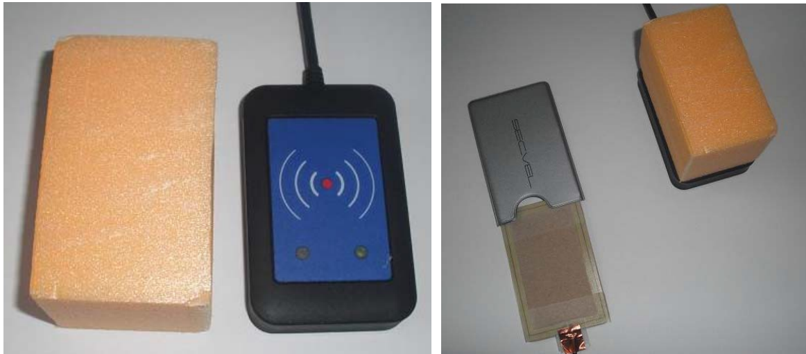
Fig. 5.6: 13.56 MHz RFID desktop reader with 5 cm separator made of rigid foam (left) and measuring antennae in the form of a bank card inserted into the SECVEL Card Protection Sleeve (right, rigid foam separator on top of the RFID reader).
