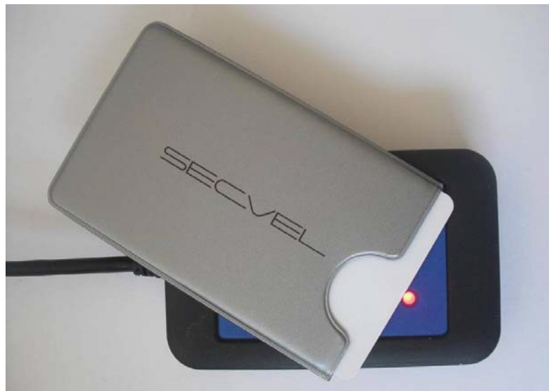
Fig. 7.4: With the card not fully inserted into the SECVEL Card Protection Sleeve , reading of the card was still possible with the desktop reader in the case of contact with the reader's surface.
